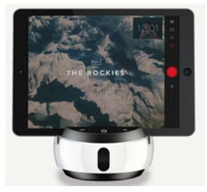
The Swivl Robot works with any tablet device and follows the movement of the marker. The marker has a built in microphone and buttons that start/stop and pause recording and tracking.
